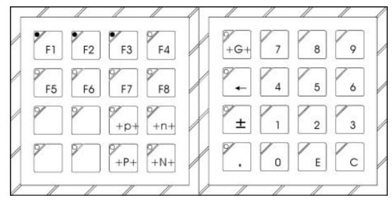
Keys F1 - F3 are assigned with key functions, i.e., specific variables in the PLC are changed when they are pressed.
